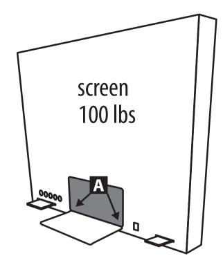
Open the hatch at the back of the screen to unscrew the 2 attachment screws (marker A).
