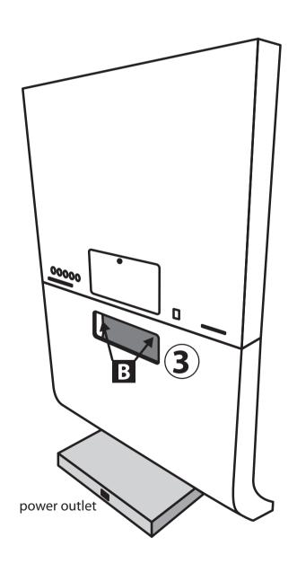
3 / Once placed the base, 1 person keeps the screen in place while the other screws in both attachment screws (marker B).
