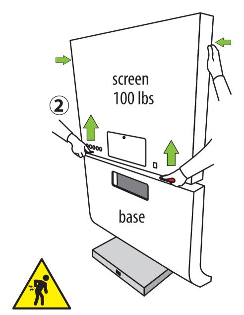
2/ Lift the screen (requires 2 people), remember to bend the legs to prevent back injuries. Careful, the screen weighs 100 lbs). Immobilize the base using your feet to prevent it from rolling and place the screen on the 2 positioning buttons.
